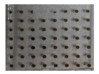
Fig. 4: The photomask B used in the photolithography of the well array
